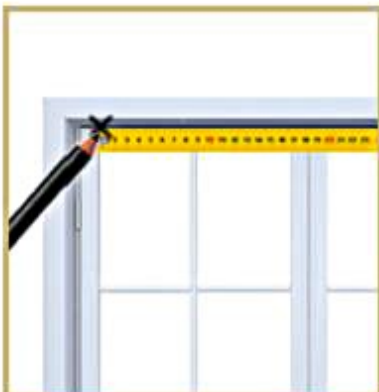
01. Measure the distance and make on the wall
