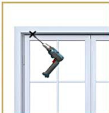
02. Drill on the wall, make sure two holes are in same level
